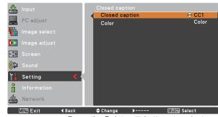
Press the Point ▲ ▼ buttons to select Off, CC1, CC2, CC3 or CC4, and then Press the SELECT button.
