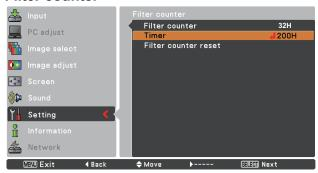
Press the SELECT button to select **Timer** and then use the Point ▲ ▼ buttons to set the timer. Select from (**Off/100H/ 200H/ 300H**) depending on the use environment.
