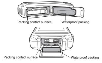
Make sure there are no foreign objects (dust, sand, hair, lint or liquid) on the rubber seals or the surface they contact before closing the battery/card and terminal covers. Wipe off any foreign objects with a clean lint-free cloth. Close the battery/card and terminal covers properly until they click.
