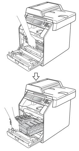
4 Turn the green lock lever (1) at the left of the machine anticlockwise to the release position. Holding the green handles of the drum unit, lift the front of the drum unit and remove it from the machine.
