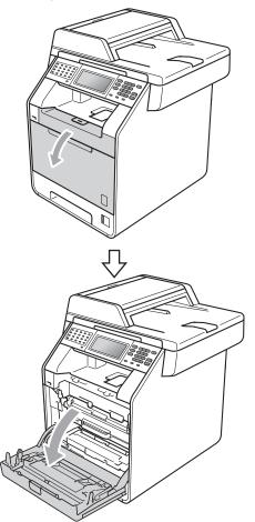
Hold the green handle of the drum unit. Pull the drum unit out until it stops.
