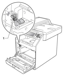
12 Match the guide ends (2) of the drum unit to the ► marks (1) on both sides of the machine, then gently slide the drum unit into the machine until it stops at the green lock lever.
