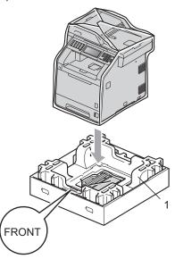
18 Put the Styrofoam piece (2) into the back side of Styrofoam piece (1) as shown in the illustration.
