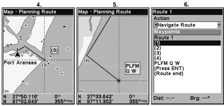
Route creation sequence, continued: Fig. 4. Point (3) set at channel mouth. Fig. 5. Waypoint (4) set further south along the beach, at a recognizable landmark (Bob Hall Pier). Waypoint PLFM Q W ends the route at an oil platform some distance from the shore. Fig. 6. Press **EXIT** to save the route and you return to this screen.
