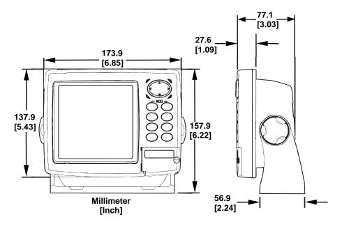
Front view (left) and side view (right) showing dimensions of Global-Map 3300C GPS unit when mounted on gimbal bracket.
