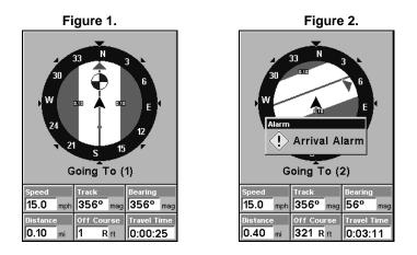
Navigating along a route: Fig. 1 shows the Navigation Page at the start of a route, heading straight for the first waypoint (Wpt 1). In Fig. 2, the traveler has arrived at Wpt 1; the arrival alarm has been triggered and the bearing arrow on the compass rose has turned to point toward Wpt 2, off to the northeast.
