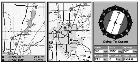
The 30-mile zoom figure at left clearly shows the red course line connecting your current position to your destination. The 30-mile zoom, center, shows both current position and direction to destination on screen. The Navigation Page, right, will also show navigation information.
