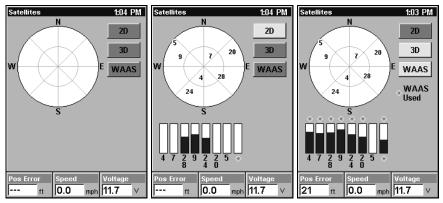
Satellite Status Page. Left view indicates unit has not locked on to any satellites and does not have a fix on its position. Center view shows satellites being scanned. Right view shows satellite lock-on with a 3D position acquired (latitude, longitude and altitude), and WAAS reception.
