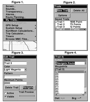
Navigate a trail menu sequence: Fig. 1, My Trails command. Fig. 2, Trails Menu. Fig. 3, Edit Trail Menu. Fig. 4, Edit Route Menu with Navigate Route command highlighted for Trail 1. A trail is always converted to a "route" when you navigate the trail.
