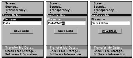
From left to right, these figures show the menu sequence for naming and saving a GPS Data File from the unit's memory to an MMC.
