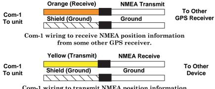
Com-1 wiring to transmit NMEA position information to another NMEA-compatible device.
