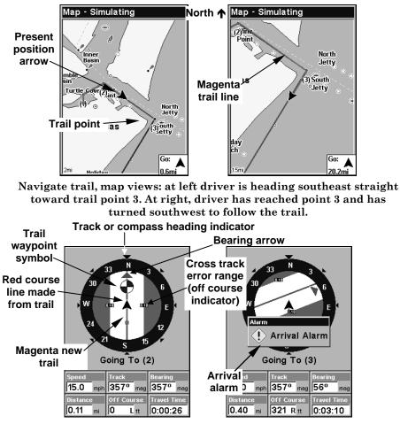
Navigate trail, navigation page (compass rose) views: At left, driver is heading north straight toward trail point 2; bearing arrow shows the trail point is 357 degrees (straight ahead.) At right, driver has reached trail point 2 and must turn northeast to follow the trail. Arrival alarm goes off and bearing arrow swings around to say turn right (east), toward the next waypoint, trail point 3. The unit now shows navigation information to point 3, which is 0.40 miles away.
