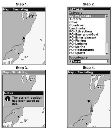
Sequence for setting a waypoint. Step 1: while traveling, *quickly* press WPT *twice* to call up Find Waypoint screen (seen in Step 2) and set a
