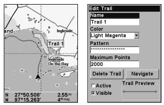
At left, trail selected with map cursor. The box at the bottom of the screen shows distance and bearing from current position to the selected point on the trail. At right, the Edit Trail menu.
