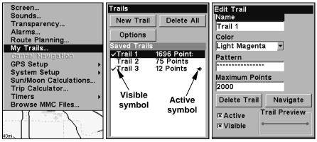
Sequence for saving a trail and beginning a new one. At left, My Trails command. Center, the Trails Menu. The arrow to the right of Trail 3 indicates the trail is "active," and the check to the left indicates the trail is visible on the map display. The right figure shows the Edit Trail menu, with the Name command selected.
