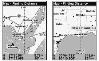
At left, the distance from the boat's current position to the cove is 5.78 miles. At right, the distance from Houston to New Orleans is 316.9 miles.
