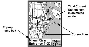
Navionics chart showing Tidal Current Station icon selected by cursor. In this example, the current is flowing to the west at 0.2 kn.
