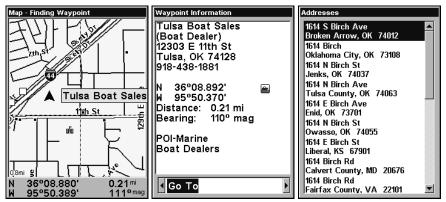
Left, Map Page showing location of the address on the map, highlighted by cursor. Center, this address is a business in the POI database, so you can display the POI information window, then navigate to it. At right, this address is not in the POI database, so the Waypoint
