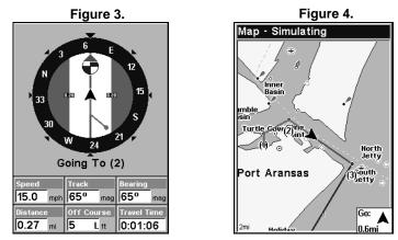
In Fig. 3 the traveler has turned northeast on his new course and is heading straight for Wpt 2, which is 0.27 miles away. Fig. 4 shows route navigation on the Map Page. In this figure, the traveler has reached Wpt 2 and is starting on the leg between Wpts 2 and 3.
