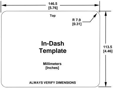
In-dash mounting template for GlobalMap 3300C GPS unit, showing dimensions. NOTE: The figure above is *not* printed to scale. A scaled template (FM-5 In-Dash Adapter Kit instructions) is available for free download from our web site, www.lowrance.com.
