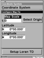
Configure a map fix so the unit can find your position on a printed chart or topographical map.
