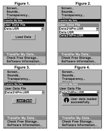
These figures show the menu sequence for loading a GPS Data File from an MMC into the unit's memory.
