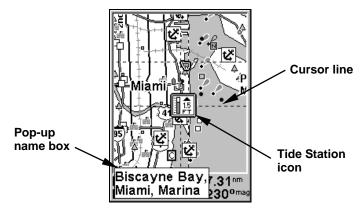
Navionics chart showing Tide Station icon selected by cursor. In the example above, the tide is at 1.5 feet and rising, as shown by the up arrow at the top of the icon.
