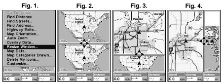
From left to right: Fig. 1. Resize Window command on the GPS Page menu. Fig. 2. Two Maps page display with four flashing arrows on the dividing centerline. Fig. 3. The centerline has been moved down to enlarge the top map, which is now zoomed in to 40 miles. Fig. 4. Pressing → has switched the page layout from horizontal to vertical – note that the relative sizes remain the same.
