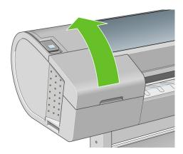
5. Press the button behind the ink cartridges to release the cover of the left-hand end of the printer.
