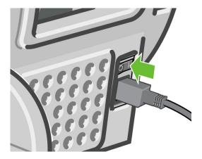
When the printer is powered back on, it takes about three minutes to initialize and check and prepare the printheads. Preparing the printheads takes about one minute and 15 seconds. However, if the printer has been off for six weeks or more, preparing the printheads could take up to 45 minutes.
