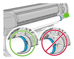
**3.** With both hands, push the spindle into both roll holders at the same time. The spindle snaps into place.
