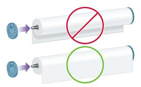
Ensure both ends of the roll are as close to the spindle stops as possible.
