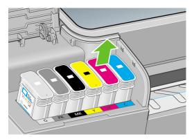
NOTE: Avoid touching the end of the cartridge that is inserted into the printer, as there may be ink on the connection.
