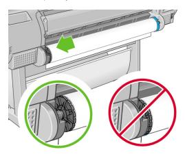
2. Rest the blue end of the spindle on the right side roll holder.
