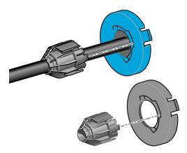
4. If the roll is long; rest the spindle horizontally on a table and load the roll on the table.
