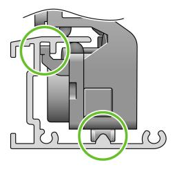
Check that the cutter runs smoothly up and down the rail. You can leave it anywhere on the rail; the printer will park it correctly later.
