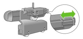
10. Slide the new cutter into position on the cutter rail.
