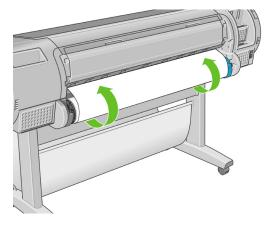
7. Once the paper is fed into the printer, the front-panel display asks if you are loading a roll or a sheet. Select **Roll** with the Up and Down keys and press OK.
