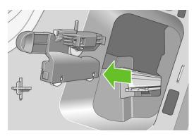
**9.** Take the new cutter from the maintenance kit and move the plunger at the top slowly back and forth within its housing to check that it moves freely.
