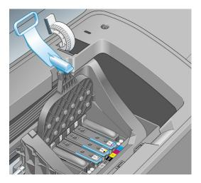
8. To remove a printhead, lift up the blue handle.
