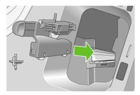
The two wheels on the bottom of the cutter should engage the central ridge on the cutter rail, and the two bushing guides should fit into the groove in the upper part of the cutter rail.
