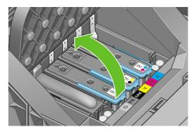
**9.** Using the blue handle, use steady force to disengage the printhead.
