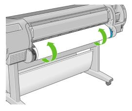
Once the paper is fed into the printer, the front-panel display asks if you are loading a roll or a sheet. Select Roll with the Up and Down keys and press OK. 8. Select your paper category and type.
