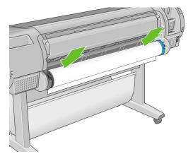
4. If the edge of the roll is not straight or torn (sometimes due to tape used to hold end of the roll), pull paper slightly beyond the cutting groove and use a cutter to cut a straight edge.
