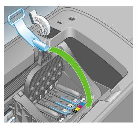
6. Ensure the end of the blue handle catches the wire loop on the near side of the carriage.
