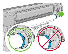
**3.** With both hands, push the spindle into both roll holders at the same time. The spindle snaps into place.
