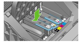
Check that you have correctly closed and latched the printhead cover, see <u>Insert a printhead</u> on page 93.
