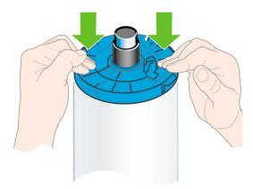
7. Ensure the blue paper stop is pushed in as far as it goes; until both ends are against the stoppers.
