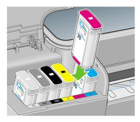
**4.** Push the cartridge into the slot until it snaps into position. You should hear a beep and see confirmation that the cartridge has been inserted.
