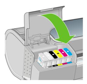
**6.** The front-panel display confirms that all cartridges have been correctly inserted, press the OK key on the front panel.
