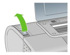
**5.** Carefully remove any of the jammed paper that you can lift up and out from the top of the printer.
