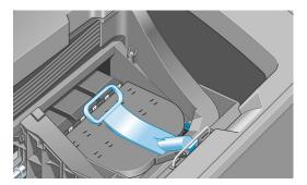
When all the printheads have been inserted correctly and are accepted by the printer, the printer beeps.
