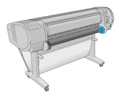
2. The spindle has a stop at each end to keep the roll in position. The blue stop can be removed to mount a new roll; it slides along the spindle to hold rolls of different widths. Remove the blue paper stop from the end of the spindle.
