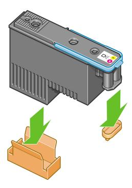
2. The printhead is designed to prevent you from accidentally inserting it into the wrong slot. Check that the colored label on the printhead matches the colored label of the carriage slot into which the printhead is to be inserted.
