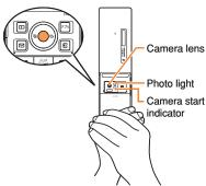
Take care not to cover the lens and optical sensor with a strap or finger.
