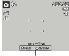
Displays the aperture and shutter speed value
