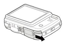
2. Open the batteries/memory card compartment at the bottom of the camera.
