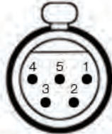
Line Audio Output Signals (5-pin mini-XLR) Connector
