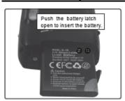
Make sure the battery has been inserted properly into your digital camera, according to the polarity shown inside the battery compartment.
