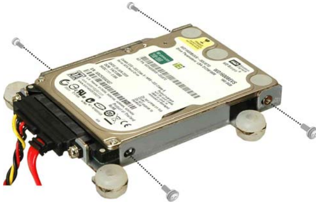
Figure 4-4: Secure the HDD with the HDD Bracket
