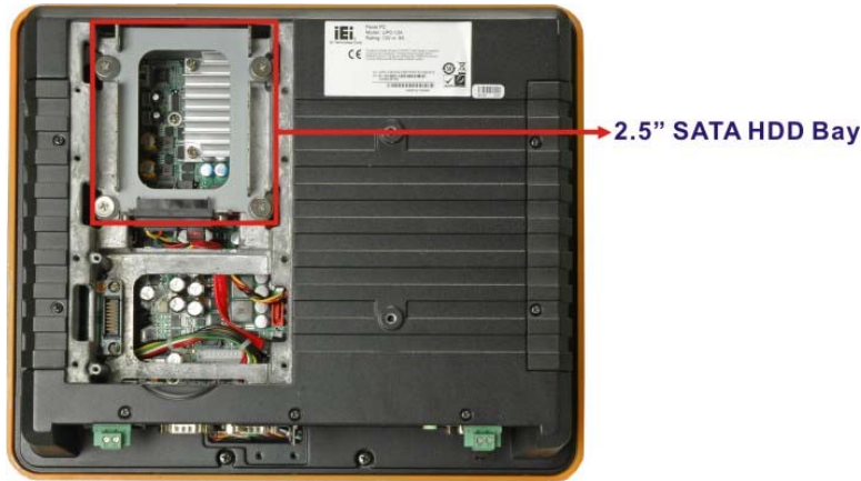
Figure 2-4: SATA Hard Disk Drive Bay
