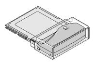
**HOW TO PUT THE PROJECTOR INTO THE STORAGE CASE** Close the lens shutter or lens cap before putting the projector in its case, then fasten the projector in place with the Velcro belt. Store the remote control unit in the remote control unit pocket, the cable in the cable pocket.
