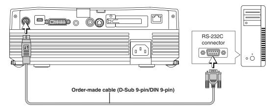
Order-made cable (D-Sub 9-pin/DIN 9-pin) pin assignment
