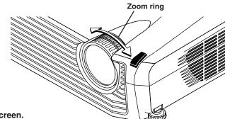
**2** Adjust the projection image to the screen. Check that the screen is set level and vertically.
