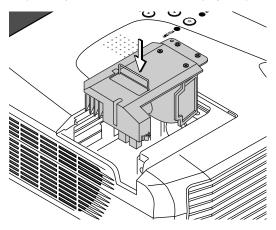
(2) Turn the two lamp cartridge screws clockwise to tighten them.
