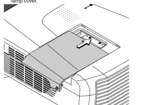
(2) Turn the lamp cover's screw clockwise to tighten it.
