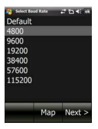
If you are using a Third-party GPS receiver on a Pocket PC or Pocket PC Phone, you can select the Baud Rate at which the GPS communicates to the software. The Baud Rate for your receiver should be listed in the packaging it came in.
