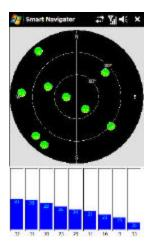
This screen displays **Satellite Information**. Typically, a nominal value of 40 or higher on at least 3 bars is normal for a GPS Lock. The bars will be gray when searching for a signal and blue when a lock is acquired. The satellites are the gray circles in the black target, which will turn green when you have a Lock.
