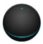
Single color pulsing slowly: The original solid color starts pulsing when setup is complete and Nexus Q is ready to use. After ten minutes, color fades to black.
