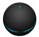
Flashing yellow: Nexus Q can't connect to Wi-Fi.
