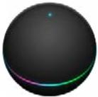
Solid color: Each available Nexus Q that hasn't yet been set up displays a different solid color, without pulsing, after successful startup.
