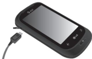
When the battery is fully discharged, you can not power on the phone. It takes approximately 4-5 minutes to reach a charge state sufficient for booting.
