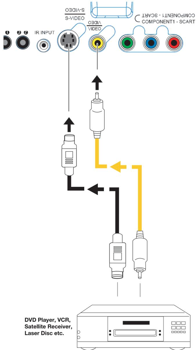
**Figure 3-13. Composite and S-Video Connections**
