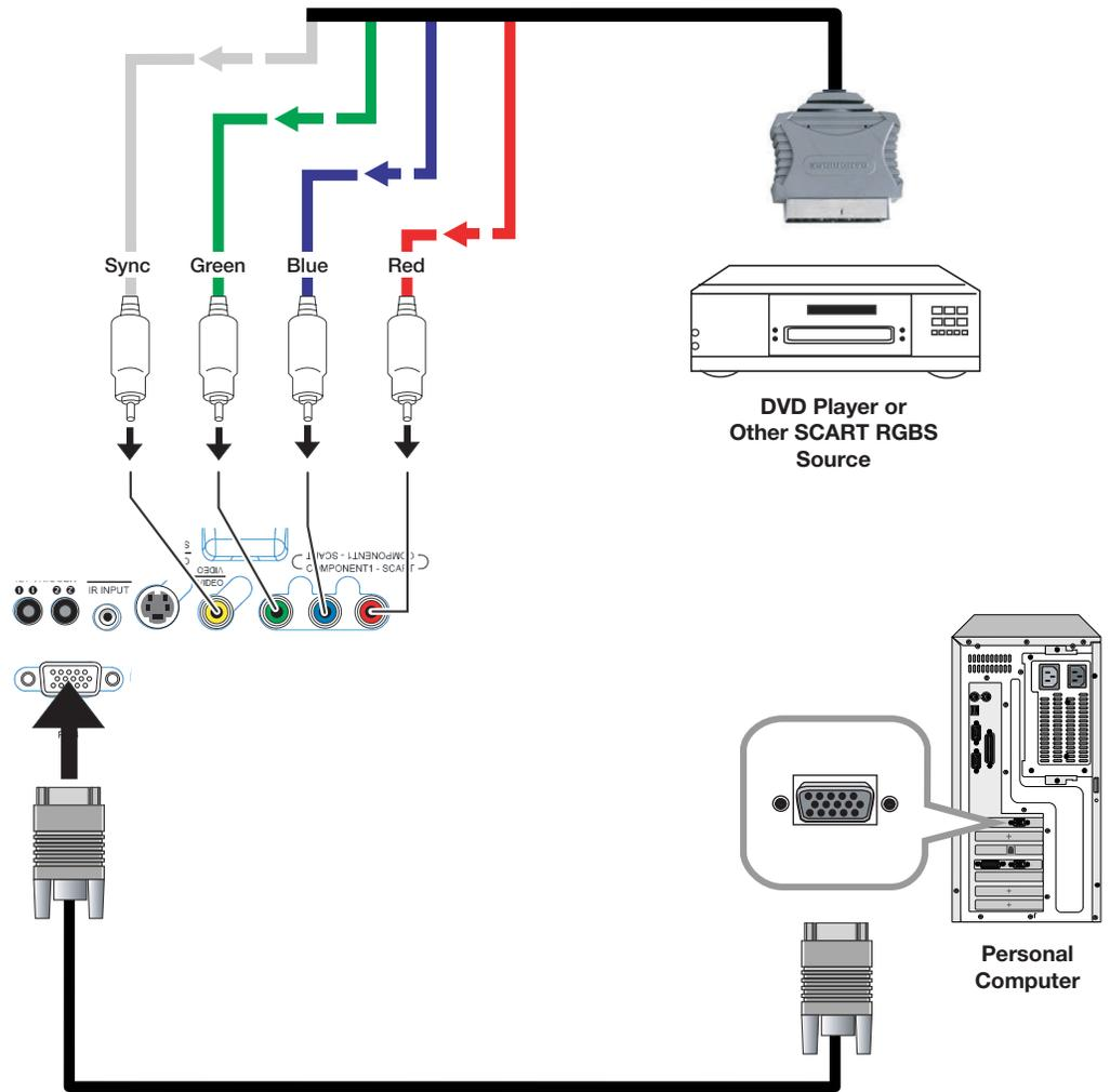
Figure 3-11. RGB Connections
