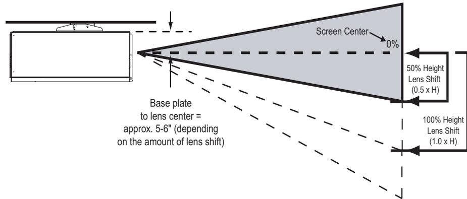
**Note:** This is a general example of lens shift. Lenses vary in their shift capabilities. **No particular lens or projector is used in this example.**
