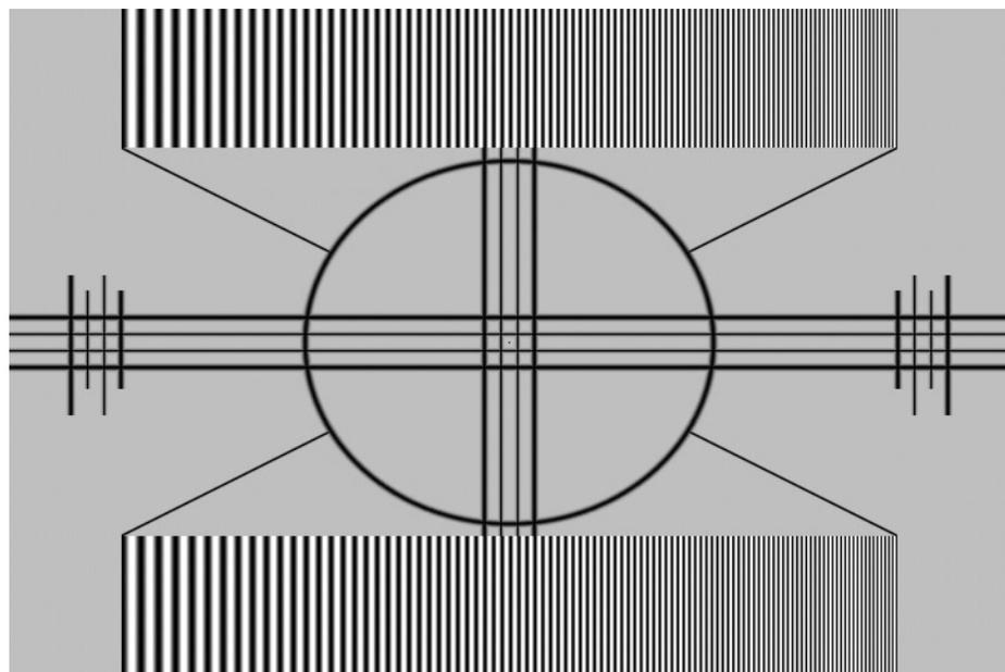
**Figure 4-5. Typical Test Pattern for Adjusting Sharpness**
