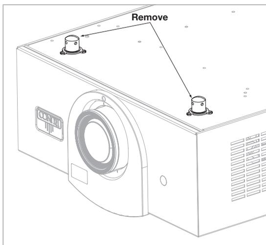
**Install Ceiling Mount Adapters/Projector Stands:** For ceiling installations, these brackets bring the mounting points for the projector mounting plate (included with the projector ceiling mount kit) from the bottom of the projector up and around the AutoScope lens motor housing. For floor installations (where the projector is upright), the adapters allow the projector to lie flat on the mounting surface.
