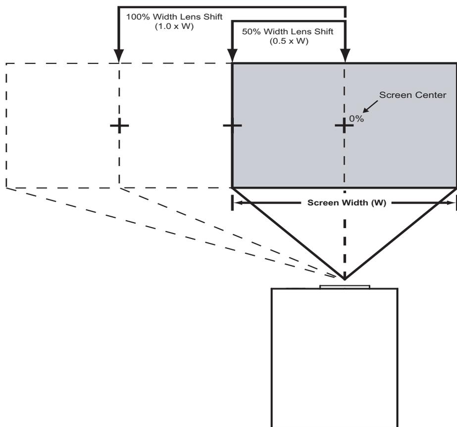
**Note:** This is a general example of lens shift. Lenses vary in their shift capabilities. **No particular lens or projector is used in this example.**
