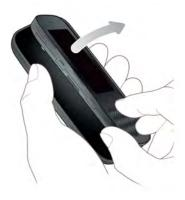
8 Remove the **battery** by sliding your finger under the groove at the side of the battery.
