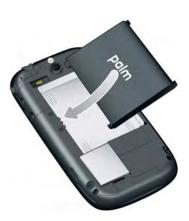
10 To replace the back cover: Insert the ringer switch into the hole provided for it on the right side of the back cover.
