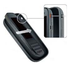
2 Press the back cover and the body of the phone together at each pair of clasps. You can feel the clasps engage.
