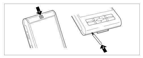
Simultaneously press the Suspend/Resume button (1) and the stylus tip (2) into the soft reset opening.
