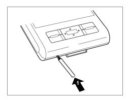
► Briefly press the stylus tip (1) into the soft reset opening.
