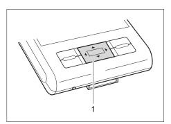
With the navigation key (1) you scroll within the menus (up, down, to the left and right) and activate menu entries by pressing the center of the navigation key.
