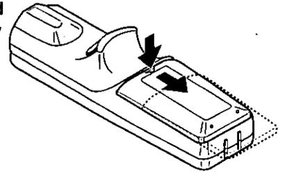
② Insert the two supplied batteries (size AA/R6). Ensure that the polarities (+ and -) of the batteries are aligned correctly.
