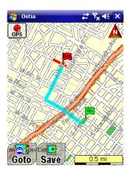
The Route will be displayed on the screen, zoomed in on the Destination. The onscreen text directions display at the bottom (if in Simulation Mode or if GPS lock is acquired). To view the whole route, tap Goto → Power User → View → Full Route. Origin displays as a Green Flag, Destination as a Red Flag, and Multi-Stop(s) as Purple numbered Flags.
