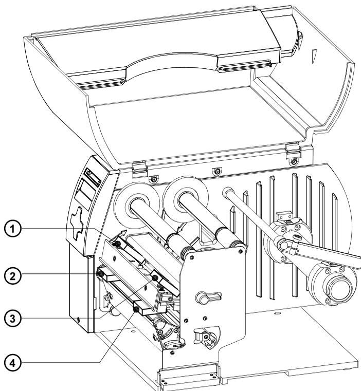
**Fig. 3** Removing the securing devices
