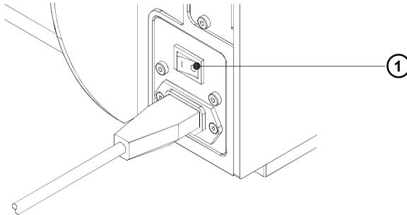
**Fig. 5c Switch on the printer**
