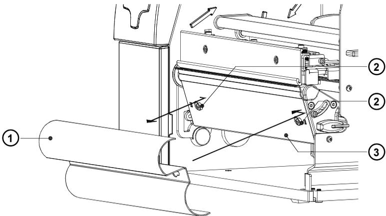
**Fig. 7b Exchange Rewind Guide Plate / Tear-Off Plate**
