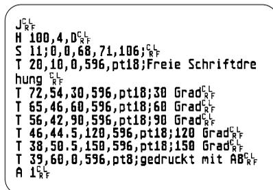
Fig. 9q Label commands printed in ASCII Dump mode
