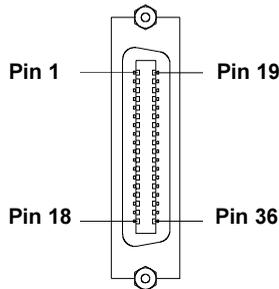
Fig. A-3 Parallel Interface Connector (rear of the printer)
