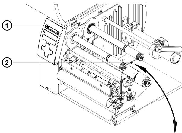
Fig. 7a Plate and warning label
