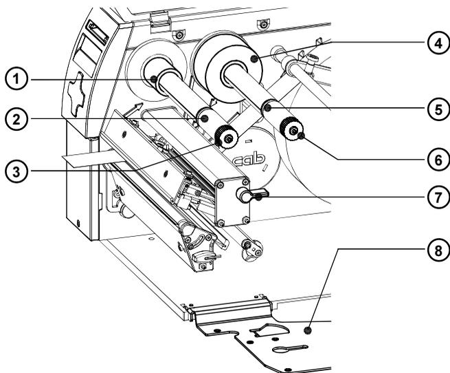
Fig. 7i Loading Transfer Ribbon
