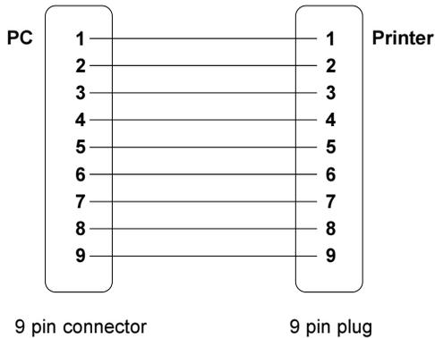
Fig. A-2 Interface Cable with 9 pin Connector
