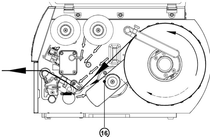
**Fig. 7d Feed path in Tear-off Mode**
