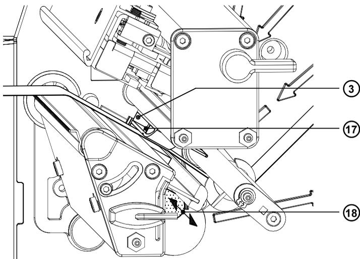
**Fig. 7e Adjustment of the Label Edge Sensor**
