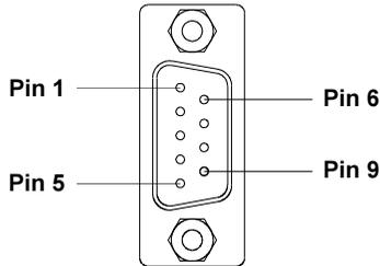
Fig. A-1 RS-232 Interface Connector (rear of the printer)
