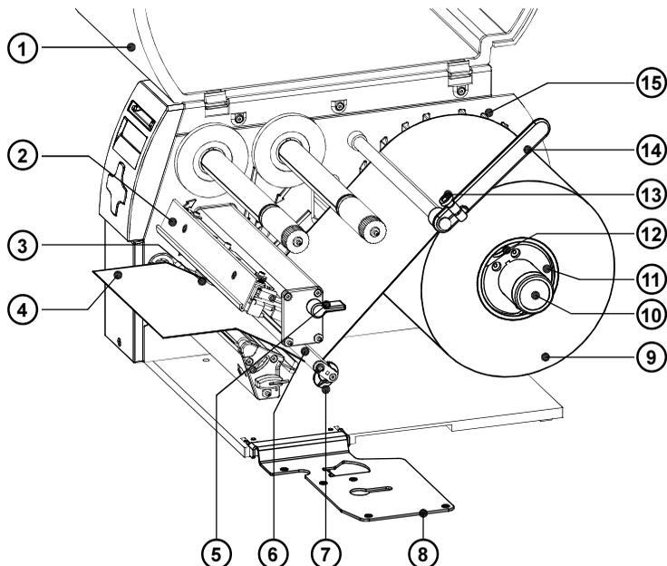
Fig. 7c Label Loading in Tear-off Mode
