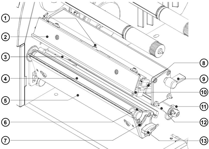
**Fig. 4b Print mechanism Basic Device with printhead open**
