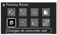
3 Press the ♣ (up), ♣ (down), (left), or CB (right) on the navigation control to highlight the Factory Reset icon, then press the center navigation control button. The Factory Reset screen opens.
