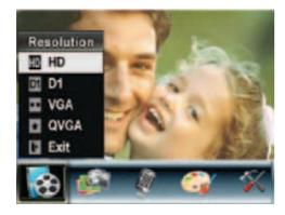
Fress T (up) or W (down) to select HD, D1, VGA, or QVGA, then press OK to save your selection and close the menu. To exit without changing the resolution, select Exit or press (Record/Play).
