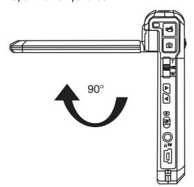
2 Rotate the LCD panel 90° counter-clockwise so you can view pictures and movies.
