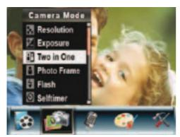
4 Press T (up) or W (down) to select Two in One, then press OK.
