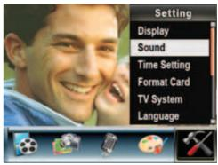
3 Press T (up) or W (down) to select Sound, then press OK. The sound setting menu opens.
