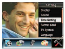
3 Press T (up) or W (down) to select Time Setting, then press OK. The Time Setting screen opens.
