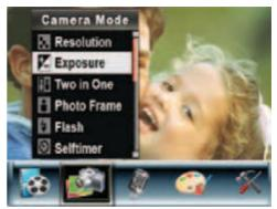
4 Press T (up) or W (down) to select Exposure, then press OK.
