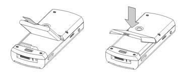
Slide the release button down and place the battery cover back in place.
