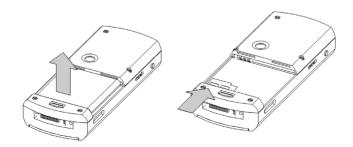
Insert the SIM card. Make sure the golden contact area is facing downwards.
