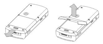
Remove battery by lifting. Pull up the locking clip.
