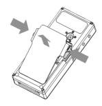
Remove battery by lifting.
