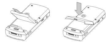
Slide the release button down and place the battery cover back in place.
