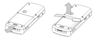
Remove battery by lifting. Pull up the locking clip.
