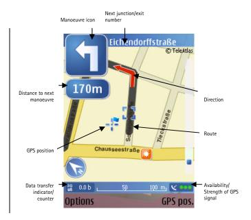
In the turn-by-turn navigation map, the route is displayed in grey. The red arrow shows the direction. The blue arrow shows your GPS position. Turns are displayed in the upper left corner and indicated through voice guidance.
