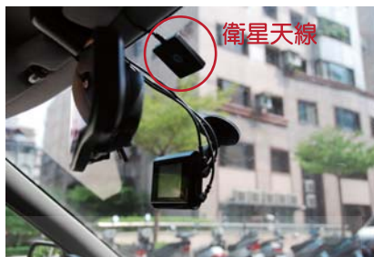
GPS antenna installation
