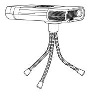
Tip: The 3M MP225 Projector will attach to most camera tripods.
