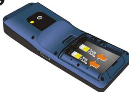
Figure 2-6: Inserting the SIM/SAM Card
