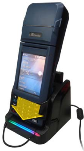
Figure 2-3: Connect the MODAT-100 to the Charging Cradle
