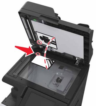
A photograph of the printer's scanning glass. A white document page is shown being placed on the glass, with a red arrow pointing to the bottom-left corner of the page to indicate the orientation. <ul style="list-style-type: none"><li>• 扫描仪玻璃用于单页文档、书页、小物品（如明信片或照片）、透明胶片、照片纸或薄介质（如杂志剪报）。</li><li>• 将文档面朝下放在有箭头的角落中。</li></ul> |
