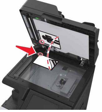
A photograph showing the scanner glass of a printer. A red arrow points to the bottom-left corner of the glass, indicating where a document should be placed for scanning. |
