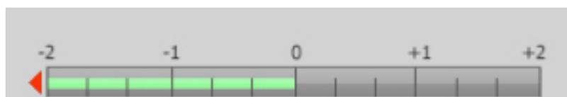
When set to program, aperture priority, or shutter priority exposure modes, the exposure meter will show a reading of about 0.0 EV. In manual, B, or T modes, you must adjust the aperture, shutter speed, and exposure compensation settings to reach a reading of 0.0 EV.
