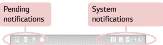
The icons displayed at the top of the screen provide information about the status of the device. The icons listed in the table below are some of the most common ones.
