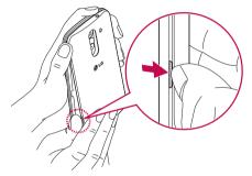
2 Slide the Micro-SIM card into the lower slot for the Micro-SIM card as shown in figure. Make sure the gold contact area on the card is facing downwards.
