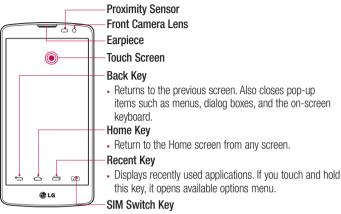
Touch the key for SIM1/SIM2 selection (Selected SIM is marked by Rectangle box on RSSI icon). Touch and Hold the key to go to Dual SIM settings.
