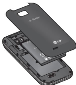
4. Align the back cover over the battery compartment (1) and press it down until it clicks into place (2).
