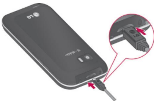
**NOTE:** Make sure the 'B' side is facing upwards when connecting the USB cable into the phone's charger/USB port.
