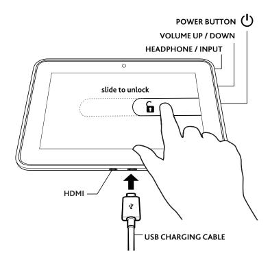
To charge your Kindle, connect it to the USB charging cable as shown. Connect the opposite end of the USB charging cable to a Kindle PowerFast accelerated charging accessory (sold separately), or other USB power adapter. To learn more about charging accessories, visit www.kindle.com/support/charging.
