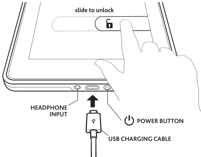
To charge your Kindle, connect it to the USB charging cable as shown. Connect the opposite end of the USB charging cable to a Kindle PowerFast accelerated charging accessory (sold separately), or other USB power adapter. To learn more about charging accessories, visit [www.kindle.com/support/charging](http://www.kindle.com/support/charging).
