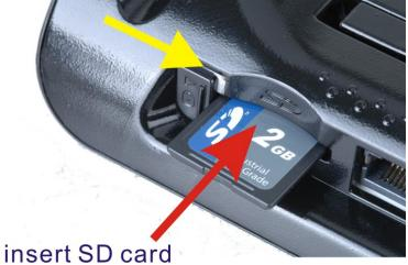
Figure 3-5: SD Card Install
