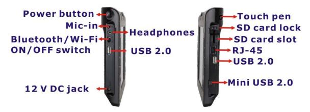
Figure 3-6: Left and Right Side I/O Connectors
