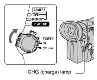
3 Connect the AC Adaptor to the DC IN jack of your camcorder. Be sure that the ▲ mark on the DC plug is facing up.
