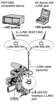
\* i.LINK jack which is compatible with HDV1080i specification is required.
