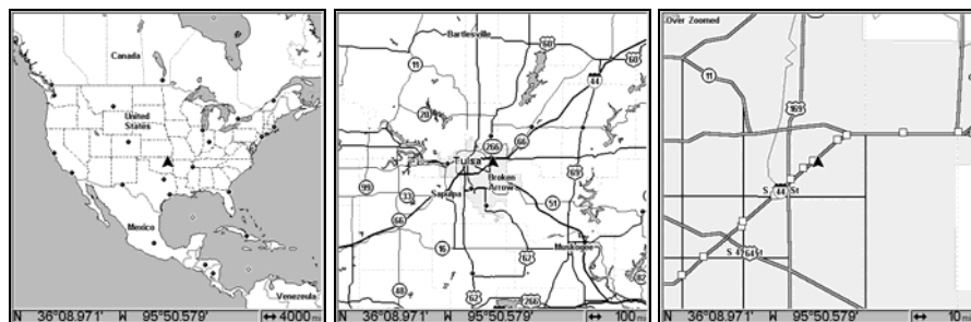
Map Page opening screen (left). Set to 100-mile zoom (center) and 10-mile zoom (right). Over Zoomed means you have reached the detail limits in an area covered only by the basic background map. Zooming in closer will reveal no more map detail because a high-detail custom map has not been loaded on the MMC for this area.
