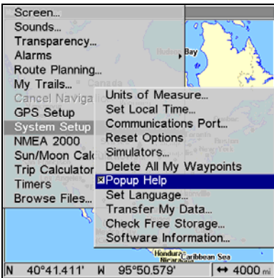
Pop-up Help command highlighted on System Setup menu (left). Pop-up Help message for Sounds (right).
