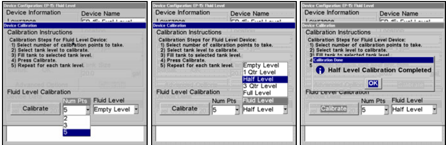
Num Pts menu with 5-point calibration selected (left). Half level selected on Fluid Level menu (center). Calibration Done window (right).
