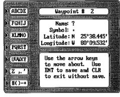
the keys on the left side of the screen. For example, to enter the name "REEF", first press the CURSOR key until the letter "R" appears. Now
