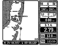
Pressing the NAV key at the bottom of the unit while the navigation screen is displayed changes all of the boxes shown at the bottom of the display. Of course, all of these displays can be changed or rearranged by the user in virtually any combination. See the Customize Screens section for more information.
