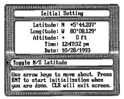
number that you wish to change. For example, to change the latitude to 41° 18.023', first press the 4 key while the "3" in the latitude is flashing. This changes the "3" to a "4". It also moves one digit to the right, making the number "6" start flashing. Now press the 1 key. Continue until all of the numbers in the latitude have changed. If you need to change the latitude
