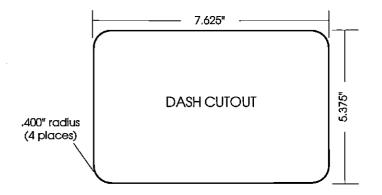
Once you've determined the location for the unit, cut the hole according to the drawing shown above. Measure carefully before cutting! After cutting the dash, place the gasket supplied with the GlobalMap 1000 around the unit and place the unit in the hole.
