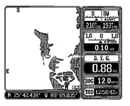
To change from the north-up to the course-up mode, simply press the MENU key, then press the key next to the "Mapping Setup..." label. Now press the key next to the "View North Up Course Up" label. This switches the check mark to the "Course Up" box. Press the CLR key to return to the
