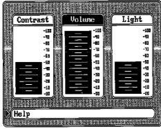
for adjustment. To change another feature on this screen, simply press the left or right arrow key to highlight the desired feature. Then press the up or down arrow keys to increase or decrease the level. When you have everything on this page adjusted as desired, press the CLR key to exit.
