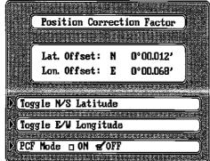
Factor (PCF) Offset feature, you make the unit read the same as the chart. If you move, the unit will continuously add the change to all position displays. This makes it more closely match the datum used by the chart. For this reason, you should be careful when entering the PCF offset. This offset is saved in memory. It doesn't change when the unit is turned off. However, a Preset does erase the PCF factor.
