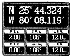
and velocity made good (VMG) beneath the present position.
