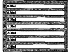
A faster way to change the C.D.I. range is to simply press the ZOOM IN or ZOOM OUT keys while the steer screen is displayed. Each time you press one of these keys, the C.D.I. range increases or decreases, depending on which key you press.
