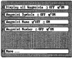
To change the waypoint display, first press the MENU key, then press the key next to the "Mapping Setup" label. Now press the key next to the "More..." label. The screen shown above appears. Press the key next to the desired option, then press the CLR key to exit this screen.
