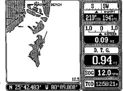
course line is always straight up, and the map rotates around your present position. Although this may look confusing at first, it actually makes reading the map easier. For example, if vou're travelling due east, features on the map should match vour view outside: an inlet on your left will be shown on the left on the map, an island on your right will show on the right on the map, etc.
