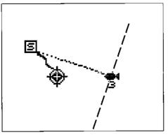
dicular to the present position's course. In this example, as soon as the present position crosses the imaginary dashed line, the perpendicular alarm will be "tripped" and sound an alarm.
