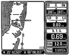
Compare the map screen shown above with the steering screen at the top of this page. The picture of the steer screen and the map screen were taken at the same time. You can see the cross track error, track, distance to waypoint, and the direction you need to steer to the waypoint easily.
