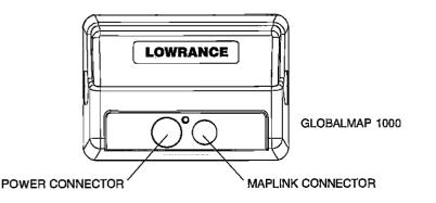
You can attach up to seven Maplink cartridge readers to the GlobalMap 1000. This lets you use different cartridges without having to unplug one and replace it with another when you move out of the first cartridge's area. This also allows the mounting of the Maplinks under the dash, out of sight.
