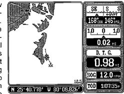
location you were in when you pressed the "Navigate to Cursor Position" label. The cursor position is marked by a small box and the letters "XX" which remain on the screen, even if you turn the cursor lines off. For more information, see the waypoint navigation section.
