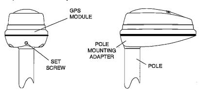
If the pole or mast you're using isn't hollow or if the hole in the middle of the pole is too small for the connectors, use the cable mounting adapter supplied with your unit. Thread the cable mounting adapter into the GPS pole mounting adapter. Then thread the pole into the cable mounting adapter. Route the cable down the outside of the pole.
