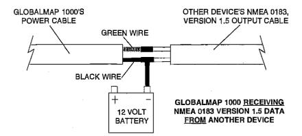
The white and green wires are for a NMEA 0183, version 1.5 interface. The GlobalMap 1000 sends data to other electronic navigation devices through the white wire and receives NMEA data through the green wire. If the white and green wires are not used, tape their ends so that they cannot short.
