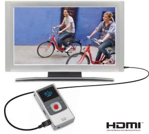
Note: You can use any brand of HDMI Cable that has an HDMI Connector (for the HDTV) on one end and HDMI Mini Connector (for the video camera)
