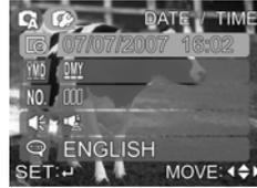
3. Use the joystick to highlight each field, and adjust the value. After the changes are done, and press the **center** joystick to confirm.
