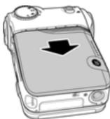
2. Insert the batteries as shown.
