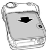
2. Insert the batteries as shown.
