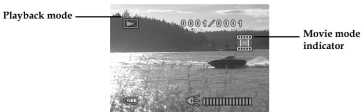
2. Press the directional pad left and right to scroll through the video clips. Press the **Shutter** button to playback the video clip.
