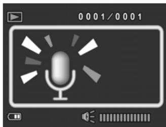
2. Press the directional pad left and right to select the voice file you want to play. Press the **Shutter** button to playback the voice file.
