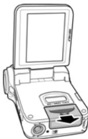
2. Insert an SD card as shown. Make sure the gold contacts are facing away from the battery.
