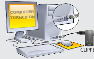
**CONNECTING/CHARGING:** When you connect the USB cable to your computer, the ARCHOS will connect as an external hard drive, for example **Clipper (E:)**, and start to charge its battery. The red LED indicator will blink while the battery charges and then remain solid once the Clipper is fully charged.
