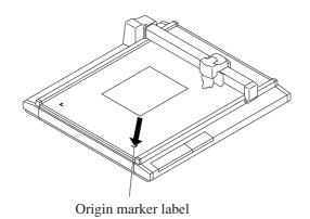
Place a sheet of A3 or larger paper in landscape orientation on the device while aligning the lower left corner of the paper to the origin marker label.
