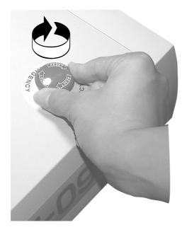
Turn the EMERGENCY button clockwise for unlocking.
