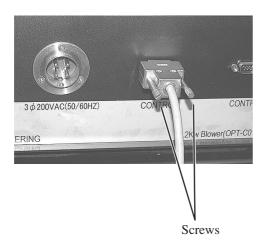
Insert the other end of the signal wire cable for the blower into the connector on the blower unit (option).
