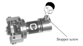
Loosen the stopper screw in the crease roller.
