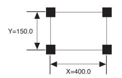
After detect the register mark, display changes to Scale compensation. If the data and detected length differs, set with (F1 +) (F2 +) key.
