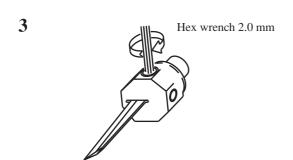
Using the supplied hex wrench (2.0 mm), fix the blade by tightening the fixing screw.
