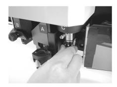
Insert the pin of unit C into the tangential cutter while fitting the pin in the groove on the cutter.
