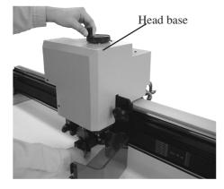
Raise the head using the height adjusting handle.
