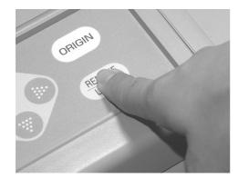
Press the (REMOTE LOCAL) key while the device is in operation.
