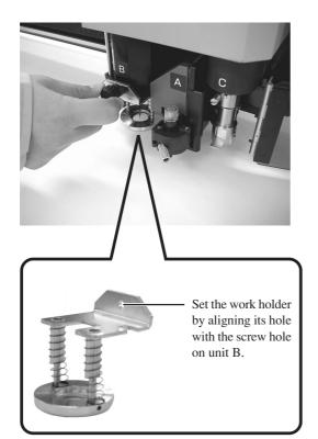
Set the work holder to unit B and tighten the screw.
