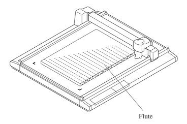
Place the corrugated board in such a way that its flutes are in parallel to the Y-axis of this device. To set a marking pressure in terms of the Y-axis direction, specify how far the pressure is reduced from the pressure value designated in the [CUTTING CONDITIONS]. See page 2.23.
