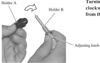
Turning the adjusting knob counterclockwise, draw out the holder B from the holder A.
