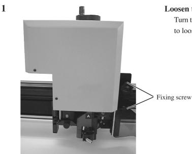
Loosen two fixing screws in the head.
