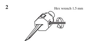
Using the supplied hex wrench (1.5 mm), fix the blade by tightening the fixing screw.
