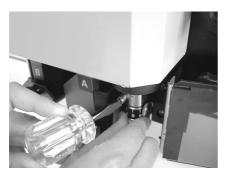
Tighten the stopper screw with the screwdriver supplied with the device as an accessory.
