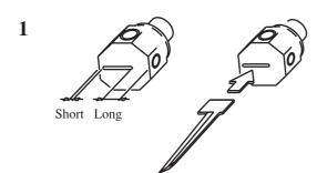
Push in the blade all the way into the cutter holder.
