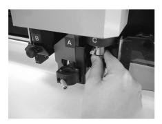
Insert the pin of unit C into the marking roller while fitting the pin in the groove on the roller.
