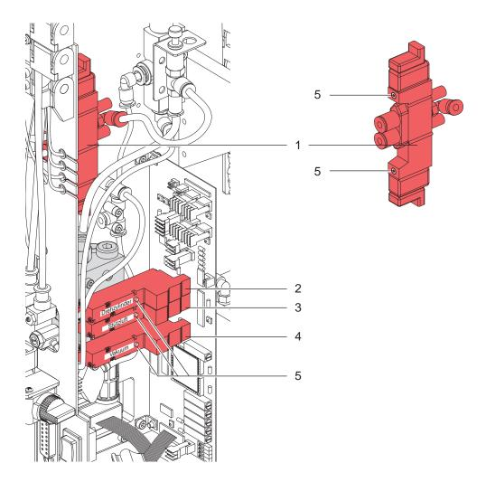
Figure 10 Pneumatic control valves
