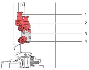
Figure 11 Throttle valve at the valve block
