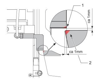
The exact adjustment of the pad in the takeover- (or start-) position is necessary to get a faultless transfer of labels between printer and applicator. To adjust the pad, put in the material like the operator's manual of the printer.
