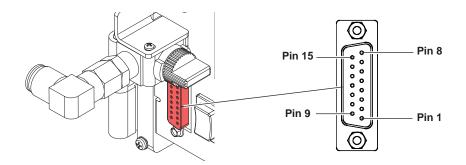
Figure 17 Female connector of the PLC interface
