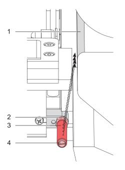
Figure 9 Adjust the blow tube
