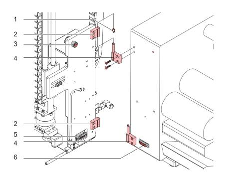
Figure 4 Mounting and connecting
