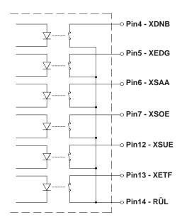
Fig. 19 Circuits of the Outputs
