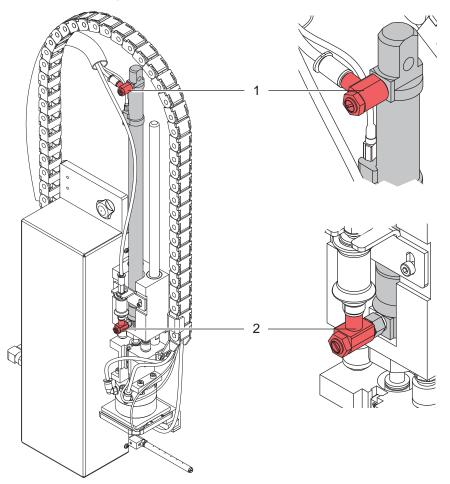
Figure 12 Throttle valve at the cylinder
