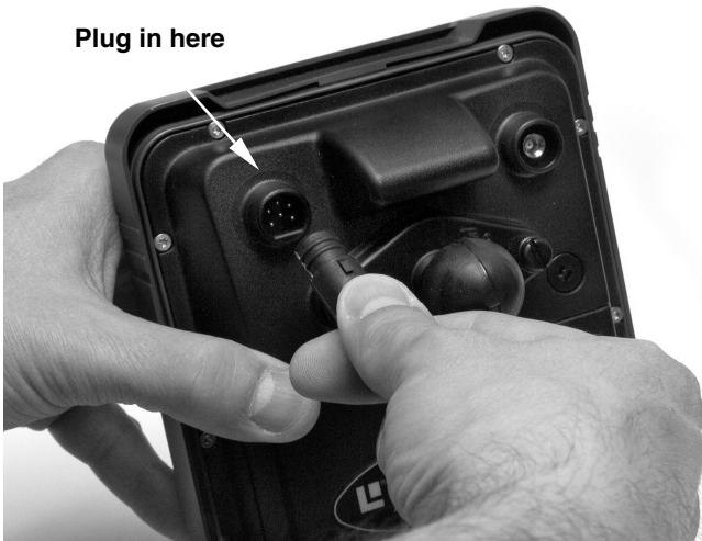
Insert the uniplug into the back of the AirMap.
