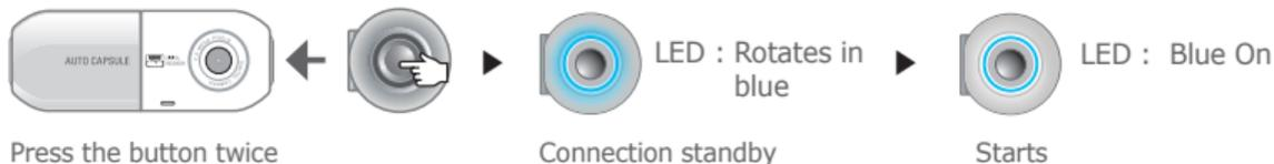
When the side button is pressed twice, the indicator LED rotates in blue alongside the voice message announcing the start of Wi-Fi connection. When the Wi-Fi connection is established, the indicator LED stays on solidly. Wi-Fi can be turned off by ending Smart Manager or pressing the button twice.
