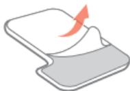
Remove the release paper from one side of the double-coated tape.
