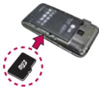
**NOTE** The microSD card can be easily damaged by improper operation. Please be careful when inserting, removing or handling it.
