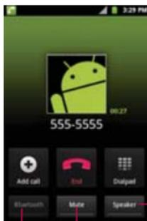
Touch to turn the speakerphone on or off. The Speaker button lights up to indicate that the speakerphone is on.
