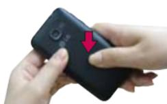
**3** Place the battery cover over the battery compartment, then press it downward until it clicks into place.
