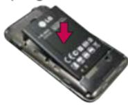
**2** Align the battery contacts with the terminals in the battery compartment and push the battery down until it clicks into place.
